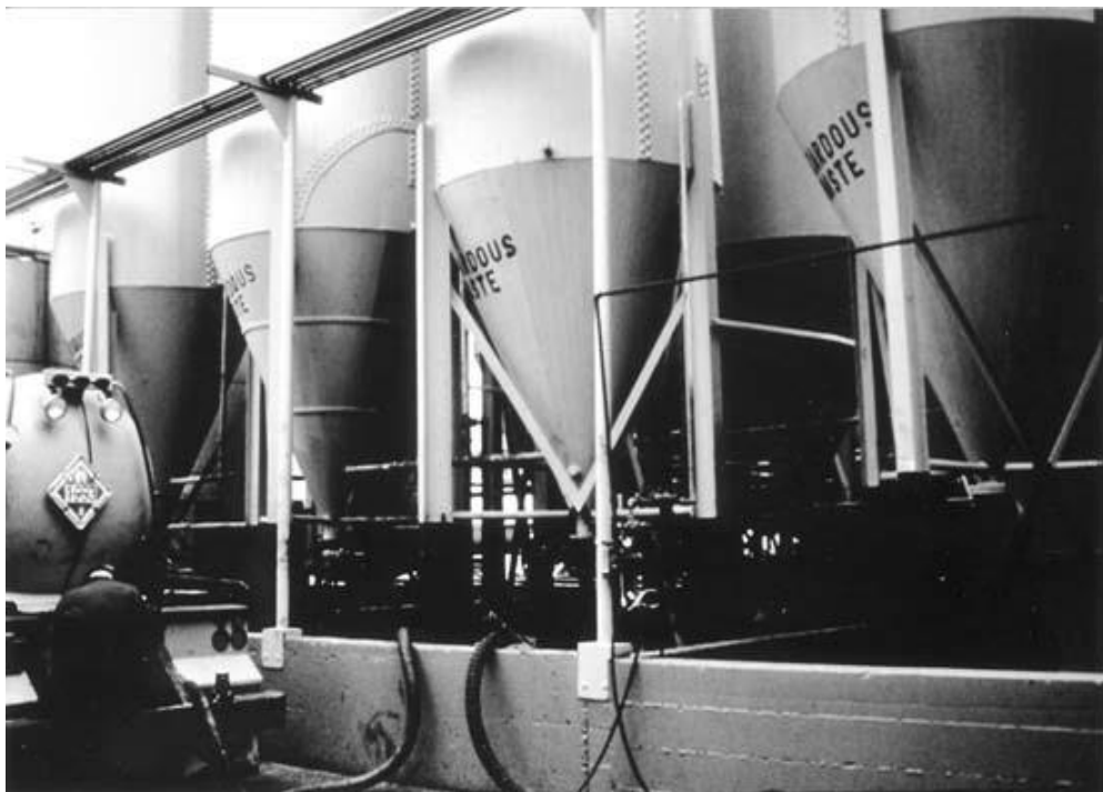
Figure 4.18 Gravity separation cones. (From ROMIC Chemical Corporation, 2081 Bay Road, Palo Alto, CA 94303. With permission.)
