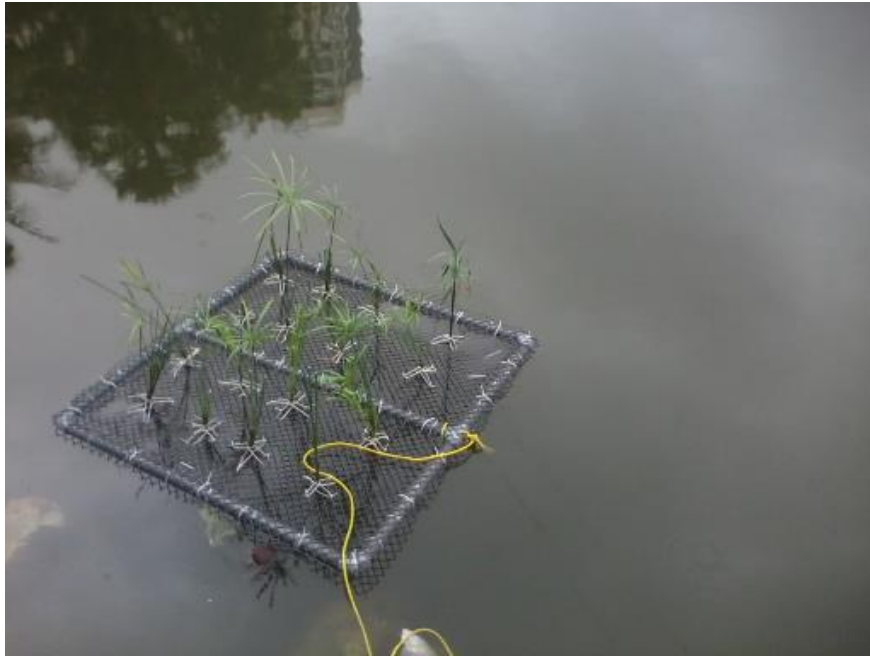
Figure 4.8: Initial Prototype of CSIR-NEERI's Floraft Technology
