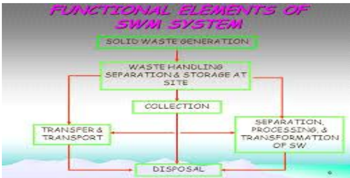
Figure 4.1 Functional elements of SWM system (Source www.slideplayer.com (ECH 4102 Environmental health engineering ppt))
