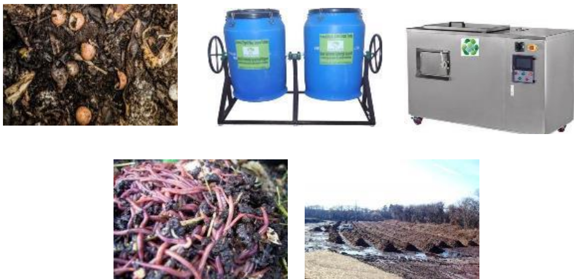
Figure 2.3: a) Composting pit b) Tumbler c) Waste composting machines d) Vermicomposting e) Windrow composting
